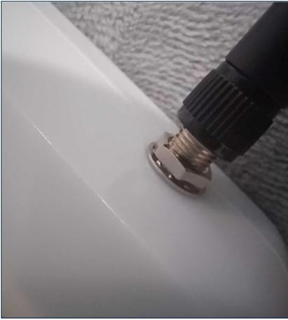
3. Attach the black LTE antenna to the small metal threaded connector on the side of the UCM by twisting it on until just finger tight. Make sure it is straight.
