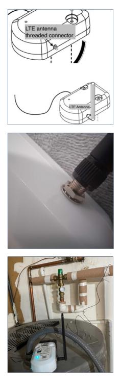
Attach the black LTE antenna to the small metal threaded connector on the side of the UCM by twisting it on until just finger tight. Make sure it is straight.
