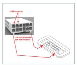
In most cases, the screw sockets on the UCM will align with the screw sockets on the CTA-2045/EcoPort<sup>™</sup> port. If this is the case, use the screws to secure the UCM to the receiver.
